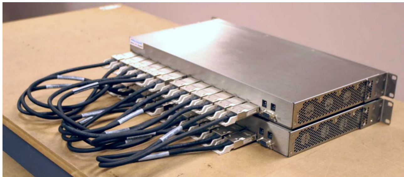
Pair of 36 Port Switches configured as a 48 Port Switch using their DDR rear ports
